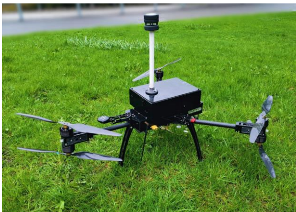
Figure 16. Mini Sniffer developed by Chalmers University
