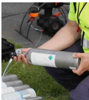
Figure 12. Daily calibration level check is always performed through the sample line in use.
