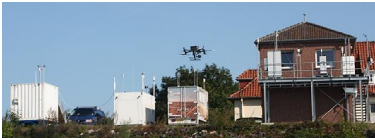
Figure 24. Setup of the side-by-side inter comparison systems at the BSH measurement site in Wedel. Left to right: Chalmers (white container and blue VW transporter car), BSH mobile measurement station (white trailer), TNO (artistic trailer), Explicit (hovering drone), BSH (elevated platform at building).
