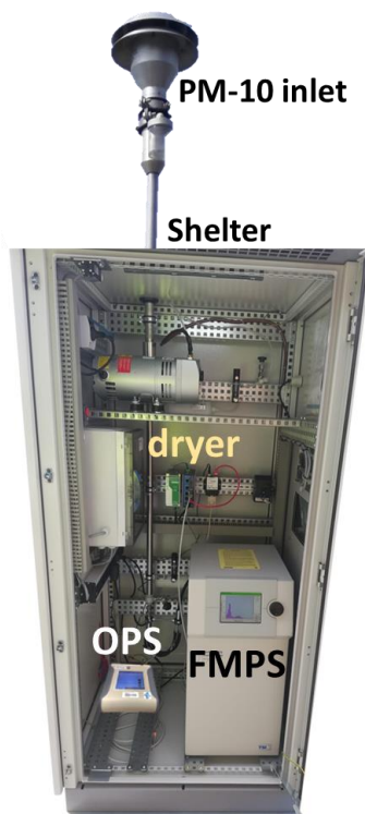
Figure 40. Combined particle size spectrometer (TSI Fast Mobility Particle Sizer + TSI Optical Particle Sizer) installed into a climate-controlled shelter. Sample air is dried with a Nafion counterflow dryer. The PM-10 inlet prevents particles larger than 10 µm to enter the system.
