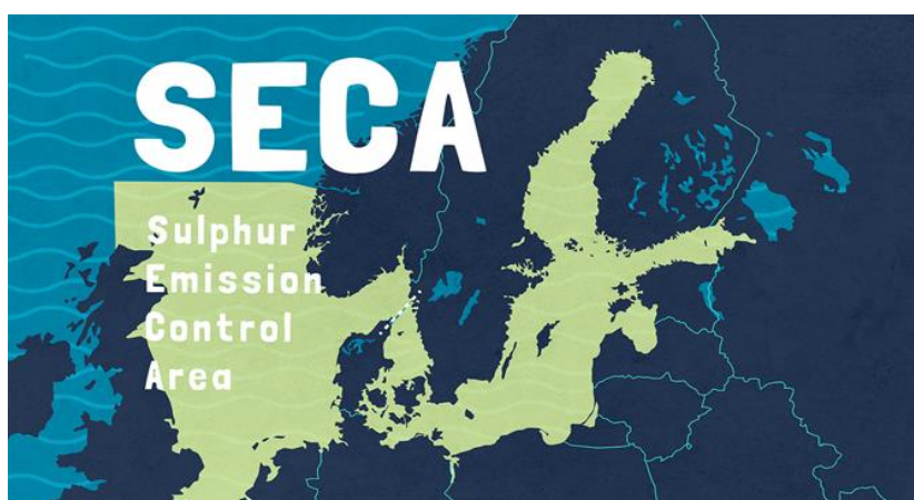
Figure 1. The European SECA area which requires fuel with FSC of 0.10% or less (for non-scrubber ships). From 2021 this area is also a NO x emission control area, requiring Tier III (approx. 75 % NO x abatement compared to Tier II) for all ships from this year and onward. The area extends all the way to 5°W in the English Channel.
